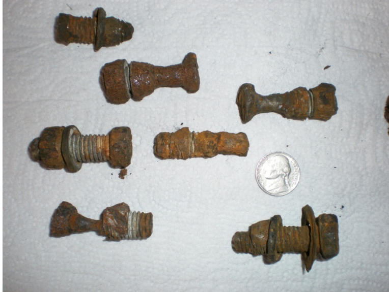
Bolts removed from the underwater structure of floating docks
